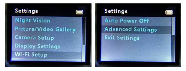
**Step 4**: In the Advanced Settings menu select "Software Version" and confirm the current software version 3.44.00 for Model #260230, 4.44.00 for Model #260240, or 5.44.00 for Model #260250 is shown below "Equinox Z2". Press the center (Select) button to exit the Settings menu.
