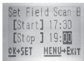
[Step 5] (opt)-set Field Scan "B" Stop & Start
