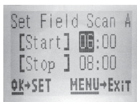
[Step 3]-set Field Scan "A" Stop & Start
