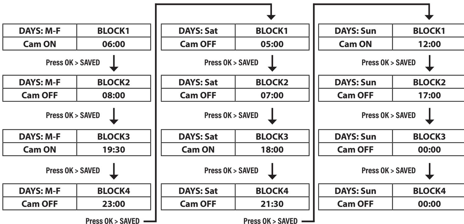
With the PIR Timer settings shown above, the result would be photos/videos that are captured (when the PIR sensor is triggered) only during these scheduled times:
