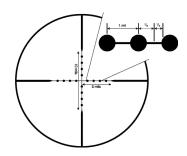
One mil is the distance between center of dots. It's easy to measure in half-mils or even quarter-mils but with practice you can measure tenths of a mil.
