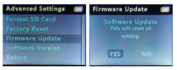
**Step 10**: Once the "Fw update" screen reaches 100% the Equinox Z2 will automatically shut off and complete the update process. Wait a few minutes, then confirm the firmware update was successful by checking the software version number, following the steps on the next page.
