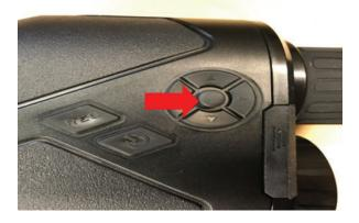
**Step 8**: In the Settings menu, press the down button (control pad button closest to the eyepiece) to navigate to the bottom of the Settings menu (the menu is continued to a second page after "Wi-Fi Setup"-keep pressing the down button). With "Advanced Settings" highlighted as shown below, press the center button to select it.
