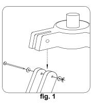
Locate the *Finderscope (1)* with pre-assembled mounting bracket. Remove the two nuts located near the front of the telescope (closet to the eyepiece) and place the *Finderscope* and bracket assembly over the exposed screws. The *Finderscope Focus Adjustment (16)* should point towards the *Primary Mirror (13)*. Replace the nuts, and securely tighten the *Finderscope* and bracket assembly in place.
