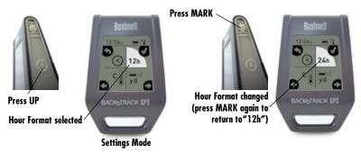
5. In Settings Mode, you may also change the other unit measurements. Press the UP or DOWN buttons to highlight the setting. Press the MARK button to change the unit measurement. You can change hour (12h to 24h), distance units (yards/miles to meters/kilometers), and temperature units (Fahrenheit to Celsius). Press POWER button to exit when done.
