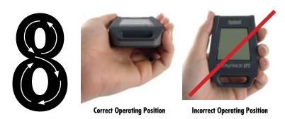
To ensure directional accuracy, hold the BackTrack out horizontally in front of you (parallel to the ground) and move it in a "figure 8" pattern a few times to re-calibrate the compass. Your BackTrack should <u>always</u> be held in a horizontal position (not tilted) as shown above when operating the unit and reading the display.
