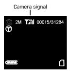
7. Prior to closing the camera, ensure the camera has acquired cellular signal. Lower signal strength can cause interruptions in service and shorten battery life. Mount the camera using the provided tree strap or 1/4"-20 mounting socket. A leveling arm to adjust the camera's angle is provided near the lower rear of the camera.
