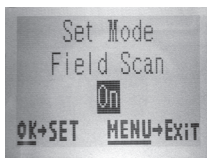
[Step 1] -set Field Scan Mode to “On”
