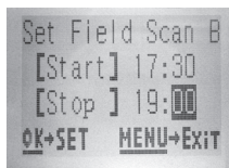
[Step 5] (opt) -set Field Scan “B” Stop & Start
