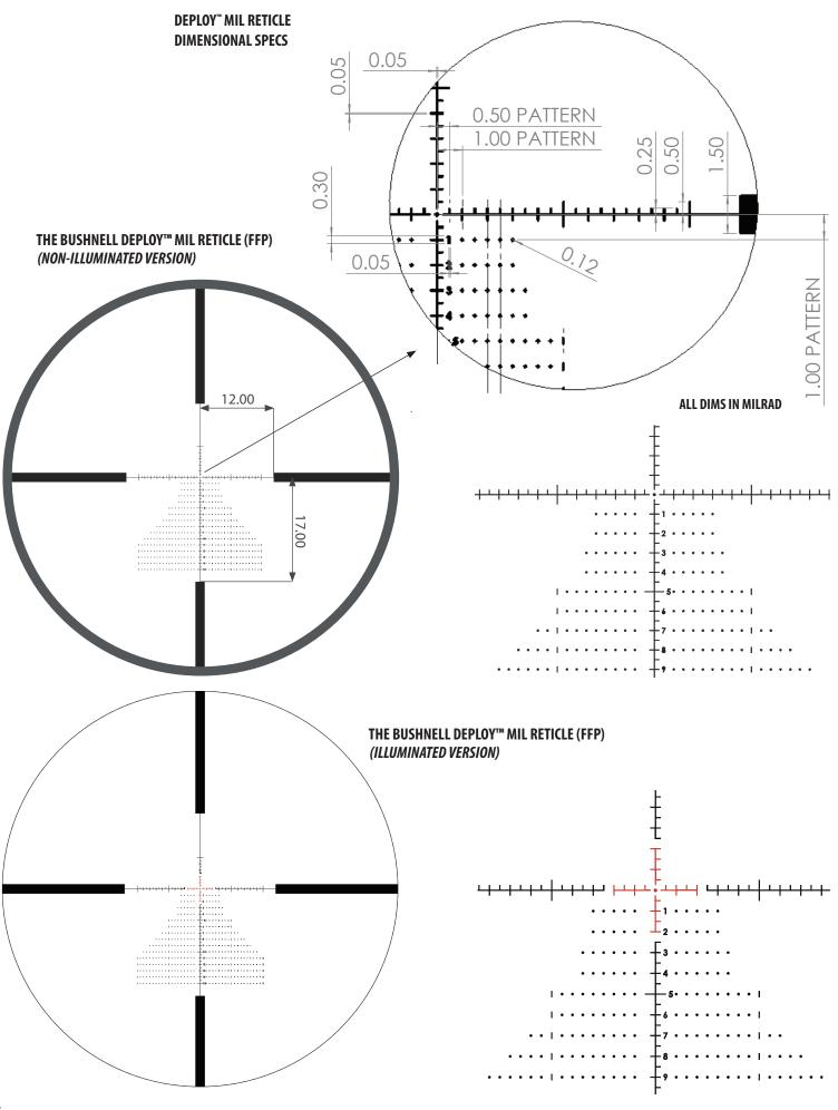
The Deploy Mil reticle is designed to be used with any caliber, bullet weight and velocity. Simply run the ballistics with a known velocity, BC, zero distance and environmental data to get your Mil drop points at various distances.
