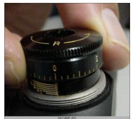
3. Retighten the Adjustment Scale Ring Retaining Screw and reinstall the Elevation and Windage Adjustment Knobs.
