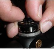
2. Lift the Adjustment Scale Ring and align the "0" with the Index Line. Be careful when setting the ring back on that you do not lose any *clicks*, which may affect your targeting at next use.
