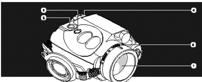
Direct the device at the subject to be viewed and adjust the final focus by rotating the objective lens focusing ring until the image quality is optimal.
