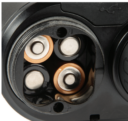
Batteries Installed (observe polarity marks inside compartment when installing batteries as shown here)
