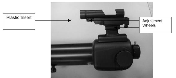
Aligning and Using Red Dot Finderscope
