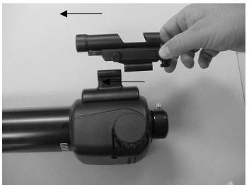
How-To-Attach: Place Finderscope Cylindrical Groove over Cylindrical Finderscope Mount Post until it clicks into place.
