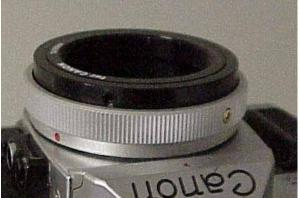
Align the red dot of the appropriate Camera Body Adapter to the red dot on the camera housing and turn clockwise until snug.
