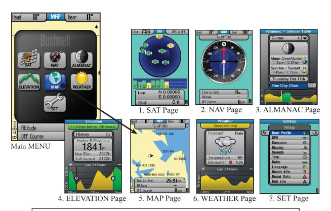
Press the MENU button briefly, use the 5-way keypad to select (highlight) a page on the menu display, then press OK (center button) to view and use that page.
