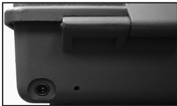
Solar Panel Input Jack
