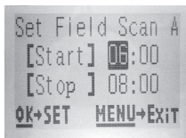
[Step 3]-set Field Scan "A" Stop & Start
