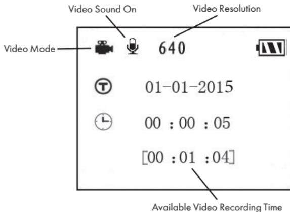
testing the camera—make sure you are in **SETUP** mode, press the **RIGHT** key, and a few seconds later a photo or video (depending on how the camera was set) will be saved to the SD card (or internal memory if no card is inserted). The “number of images taken” counter on the bottom left of the LCD will increase by one. If the display indicates “SD PROTECTED” when you press the SHOT key, switch the camera OFF, remove the SD card and slide its protect switch off.
