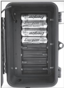
of the **Trophy Cam HD**, making sure that the polarity is correct. *Note: The power connector is a 4.0x1.7mm coaxial DC power plug with positive “tip” (inside pin) polarity (Radio Shack P/N 274-1532 or equivalent).*
