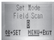
[Step 4] (opt) -select Field Scan "B" (press OK)
