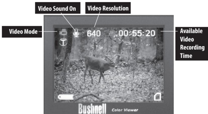
*\* Only still photos can be transmitted wirelessly, due to the large files generated by video and carrier bandwidth limitations. When the camera is set to video mode, the video files are stored on the SD card for later review (see PLAYING BACK/DELETING THE PHOTOS/VIDEOS, pg.42)*
