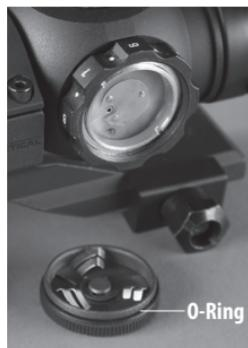
**Note:** before installing the Battery Cap, verify that the O-ring is present (see photo above) and not damaged. Failure to do so could result in water leakage into the battery compartment.
